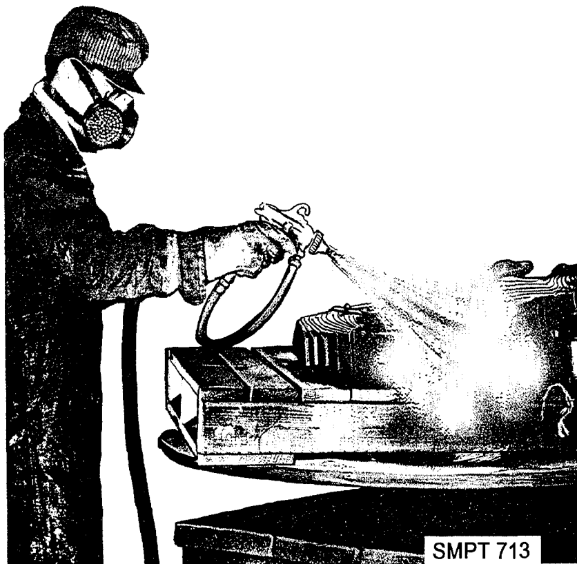
Figure 3-10. Application of preservative by spraying.
