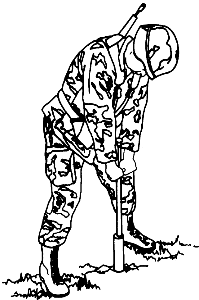
Figure E-8. Operating the remolding test equipment to obtain a soil sample
