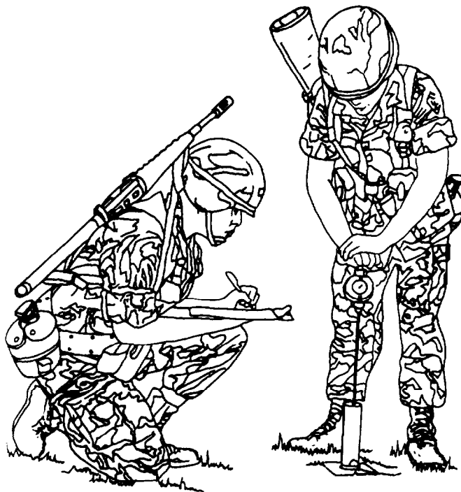
Figure E-10. Measuring cone index in a remolding cylinder
