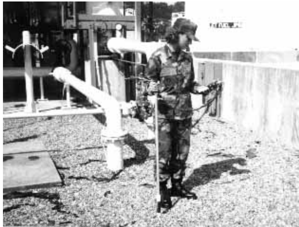
Figure 1.1. Using Data Logger for Close Interval Survey.
