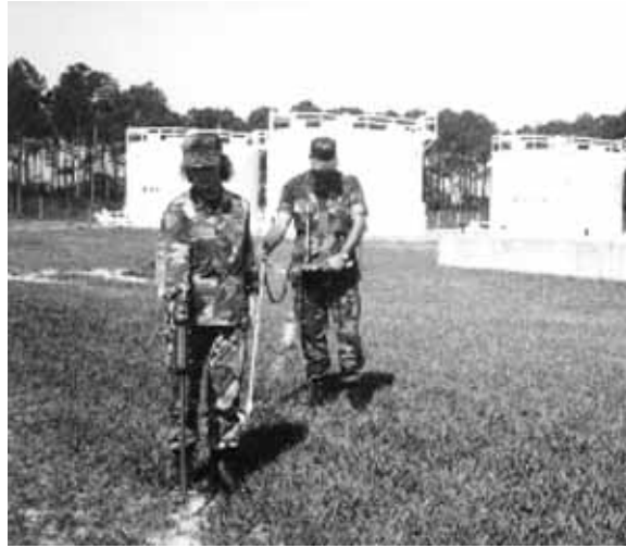
Figure 1.2. Using Pipe Locator to Make Measurements Directly Over Pipeline.
