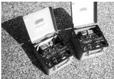
Figure 1.3. Synchronizing Current Interrupters.
